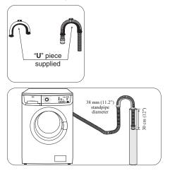
Firstly form a hook in the end of the drain hose using the «U» piece supplied. Place the drain hose into your standpipe, which should have an internal diameter of approximately 38mm thus ensuring there is an air break between the drain hose and standpipe.
